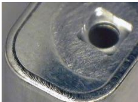
Seam weld example
