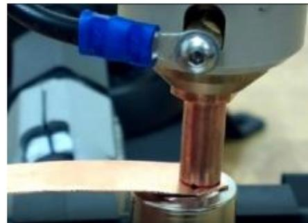
0.3 mm copper tab to 18650 battery cells
