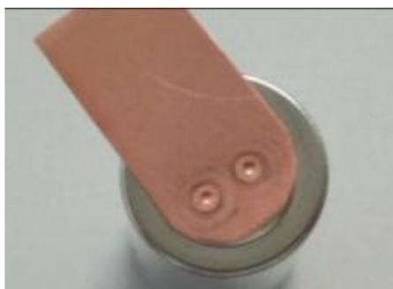
Welding 0.3 mm copper tab to battery cells
