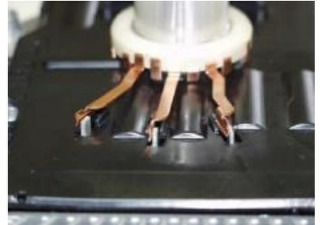
Projection Weld Radiator Connector
