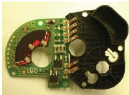
Resistance Weld Engine Component
