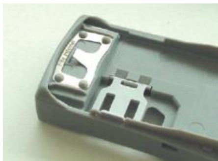
Heat stake thermode application mobile phone heat staking
