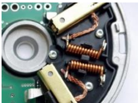
Welding stranded wire to terminal
