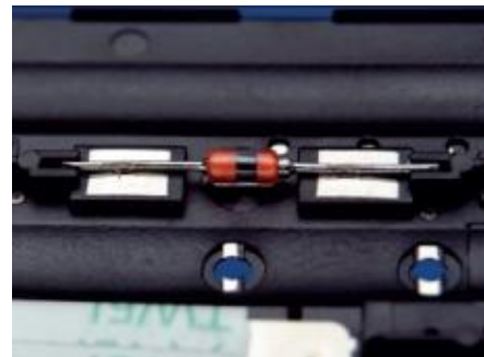
Welding components to leadframe
