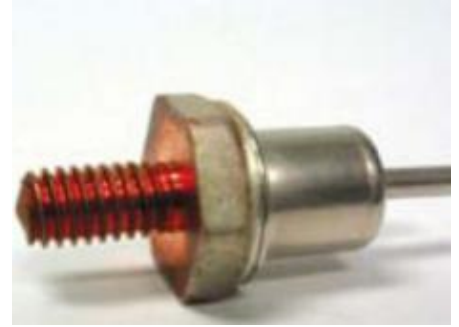
Projection welding of electronic components
