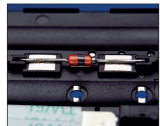
Welding components to leadframe
