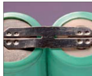
Welding tabs to batteries
