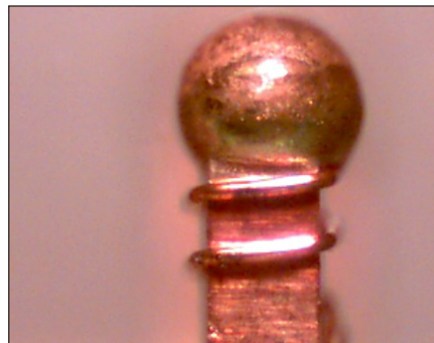
Insulated wire wrapped around a terminal pin
