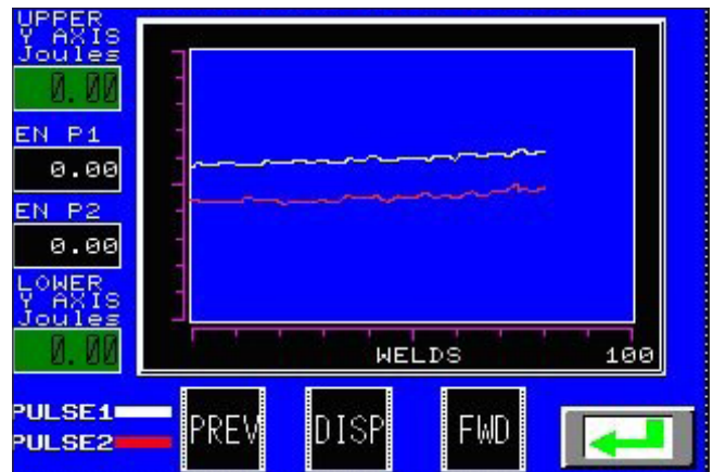
Energy trend plots indicate process performance and electrode life over time
