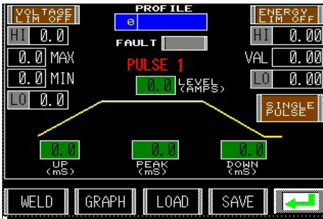
Programming screens provide 99 stored profiles, each graphically programmable via the colour touch screen.
