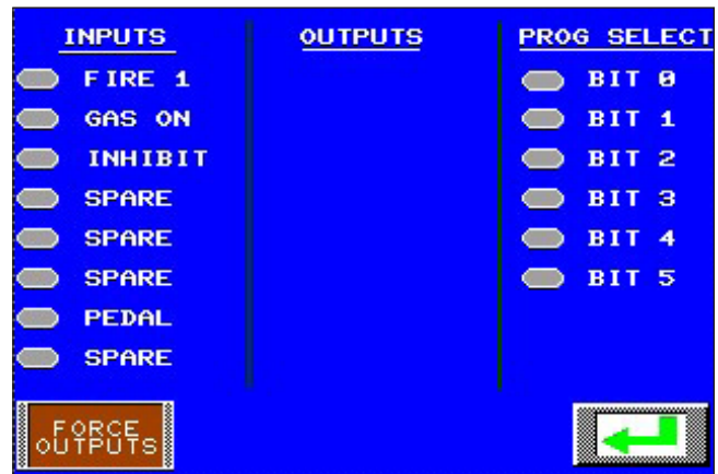
A graphical input/output monitor provides simple setup vof diagnosis of automation connections.
