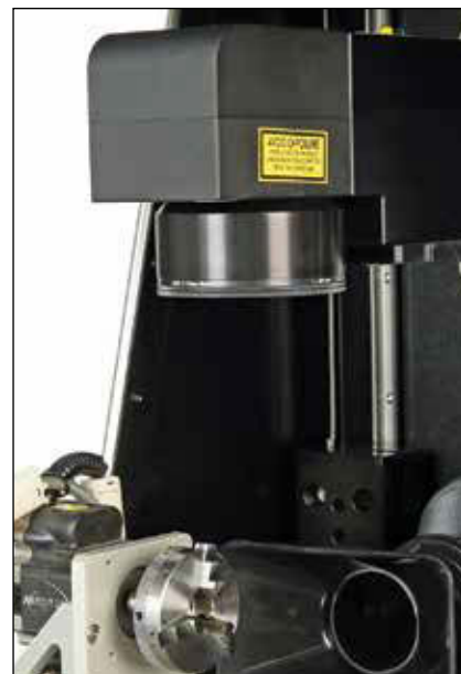
View of workspace including Z and rotary axis, fume extraction, and optical breadboard
