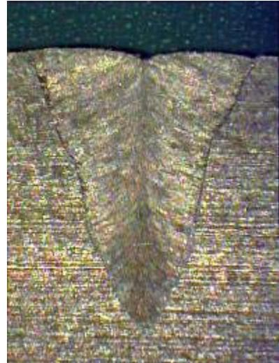
Picture 1: Seam weld, standard keyhole welding
