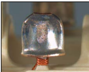
Figure 3. Welding Application - Enamelled Copper Wire on Square Pin. Wire diameter 70 \mu\text{m} .
