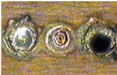
FIGURE 1. Typical spot welds on bare copper using a 1064nm and 532nm pulsed Nd:YAG laser.
