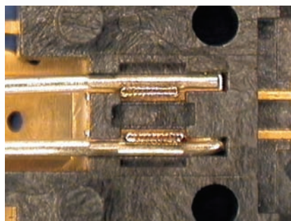
FIGURE 3. Small seam weld between 0.016 x 0.09 in. gold-plated copper lead and 0.016 in. diameter silver-plated copper wire.
